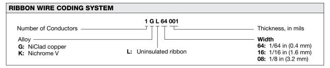
The Wire and Cable Coding System shown above gives the unique designation of each wire type for ordering purposes. The leadwire and cabling selection charts presented on the next three pages are organized according to the number of conductors. All wires and cables are supplied on spools for user convenience. Some styles may not be continuous length.
