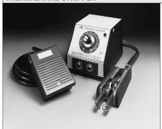
The ease and simplicity of operation of the Thermal Wire Stripper make it ideal for most strain gage leadwire stripping. The variable heat control allows stripping of all thermoplastic insulations, including Teflon®, in sizes No. 18 to No. 36 AWG (1 to 0.1 mm diameter). The foot switch and tweezer hand- piece give excellent operator control over the stripping operation. Includes power unit and foot switch, both with 3-wire NEMA plugs, and tweezer handpiece.
