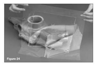
leaving approximately 1/8 in [3 mm] extending beyond the edge of the structure. Final trimming can be done after full polymerization (see Application Note B-223). If small air pockets form under the plastic, carefully lift the edge of the plastic sheet up to the air pocket and, with oiled fingertips, smooth back the plastic, pushing the air pocket to the edge of the sheet.
