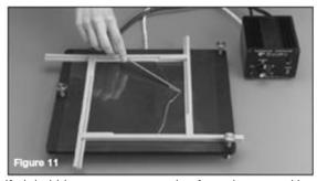
If air bubbles are present, wait a few minutes and burst them with a dental probe or a similar pointed object. Replace the cover over the casting plate.
