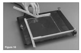
last procedure may require holding down the Teflon carrier at the same corner. In the same manner, remove the adjacent rubber frame section (see Figure 16).
