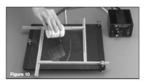
DO NOT scrape excess plastic from the cup sides and bottom onto the casting plate, as these are areas where a non-uniform mix is most likely to occur. As illustrated in Figure 11 on page 6, the stem thermometer or a wooden tongue depressor may be used to help spread the plastic over the entire plate surface (the liquid will level with time). Place the cover over the poured sheet to protect it from dust and other foreign matter during polymerization and switch the temperature controller off.
