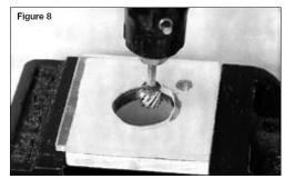
high speed and slow feed is a good general rule. The bit should be backed out of the hole frequently to clear the chips and avoid unnecessary friction. A drill press may be convenient for flat sheets; however, irregularly shaped contour sheets can make the drill press impractical.
