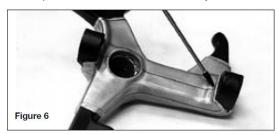
2.4 Tools and Methods Used to Machine PhotoStress Plastic Coatings\* Saber saws, coping saws, hand drills, abrasive paper, and hand routers are common hand tools normally used to machine and trim plastic coatings to the geometries discussed in Sections 2.1, 2.2 and 2.3.
